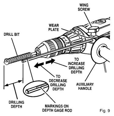
When drilling holes with the depth gage rod installed, the desired hole depth has been reached when the end of the rod comes in contact with the surface of the material being drilled.
